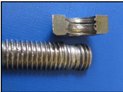
Figure 1 – Thread Galling Example
